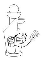
Insert the water pump into water tube.
