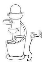
Connect the power cable to the outlet. If installed correctly water should flow from the fountain. On first use the potentially could have air in the pump so, it makes take a few minutes until the air escapes.
