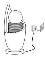
Connect the power cable to the outlet. If installed correctly water should flow from the fountain. On first use the potentially could have air in the pump so, it makes take a few minutes until the air escapes.
