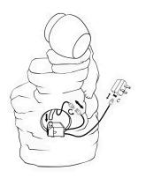
Insert the water pump into water tube.
