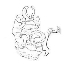
Connect the power cable to the outlet. If installed correctly water should flow from the fountain. On first use the potentially could have air in the pump so, it makes take a few minutes until the air escapes.
