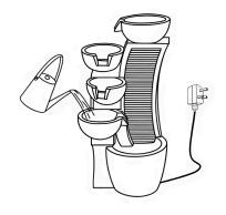
Add water so that the pump is submersed in the water.
