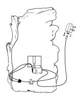
Insert the water pump into water tube.
