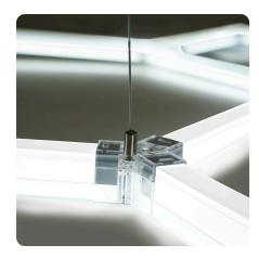
Now, start forming each hexagonal shape by connecting the 440mm LED tubes with 120° and 360° Y two-way connectors according to the pattern you desire. Ensure a 360° Y two-way connector is installed on the corner of one hexagon to allow for the second power cable connection.
