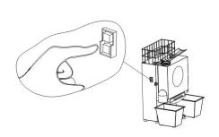
Press the start switch so the Juicer begins to feed the oranges into the juicing mechanism. Once the juicer has completed it will release the juice at which point the fruit peel will be automatically separated into the fruit peel bucket.
