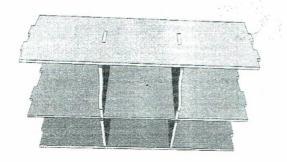
Place panel D on top of the two G panels. Once positioned secure with screws.
