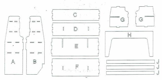
Note this unit is designed to work on either side of the van on top of the wheel arch. Looking at the unit from the front if fitting to the driver side of the van make sure panel B is on the left-hand side. If fitting to the nearside of the van make sure that Panel B is on the right hand side of the unit.
