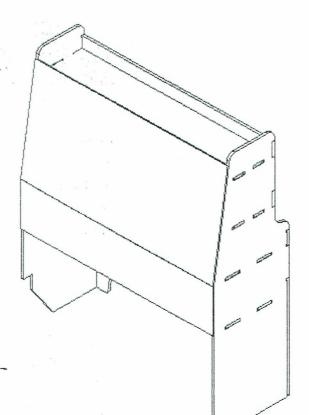
Fit the J strips fit into the recesses on the front, these are screwed to the shelves to form a retaining lip.
