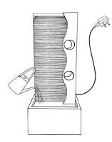
Add water so that the pump is submersed in the water.
