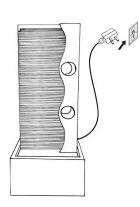
Connect the power cable to the outlet. If installed correctly water should flow from the fountain. On first use the potentially could have air in the pump so, it makes take a few minutes until the air escapes.
