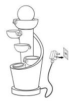
Connect the power cable to the outlet. If installed correctly water should flow from the fountain. On first use the potentially could have air in the pump so, it makes take a few minutes until the air escapes.
