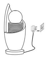
Connect the power cable to the outlet. If installed correctly water should flow from the fountain. On first use the potentially could have air in the pump so, it makes take a few minutes until the air escapes.
